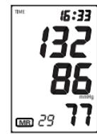
30 sets of stored measurements – MR30: Value of the last measurement – MR29: Value of the measurement before MR 30
